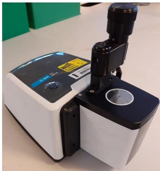
Figure 5a and 7b: the mini ATR seen from above and in perspective
