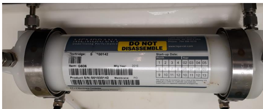
Figure 5 - Porous membrane for oxygen removal
