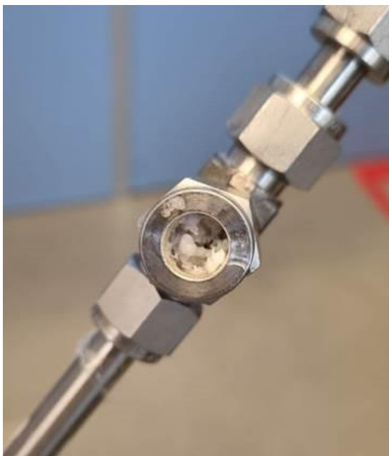
Figure 12 - Crystals observed on the gas outlet of the dense layer membrane
