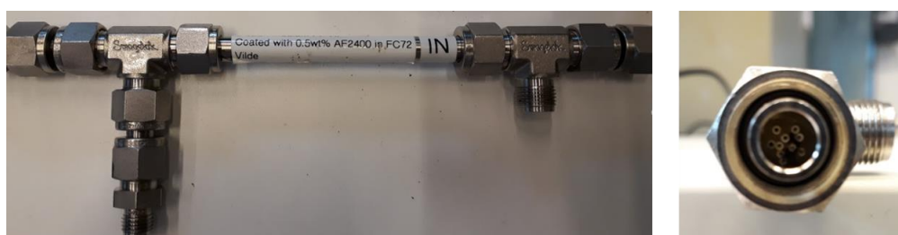
Figure 6 - Dense layer membrane for oxygen removal
