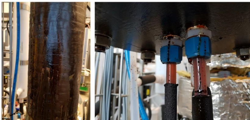
Figure 5, leakages in the non-metallic capture rig, both in the stripper column and connections to the reboiler.
